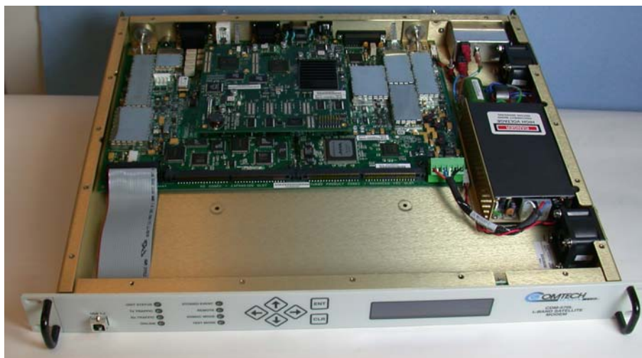
Figure 1. MPP50 properly installed in the CDM-570L modem (full view of inside of chassis)
